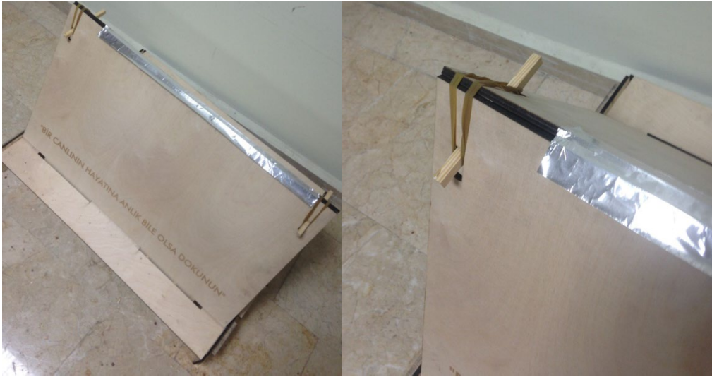
Figure 11. Team-7 Testing mock-up solutions for water leaking problem
