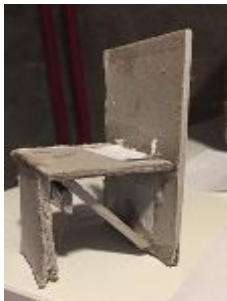
Figure 8. The use of paper strips to fix connections
