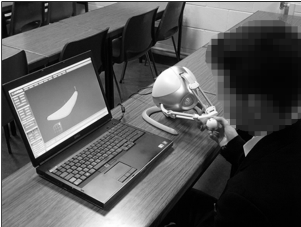
Figure 1. A participant using CRE8 and the Novint Falcon to model an organic geometry.
