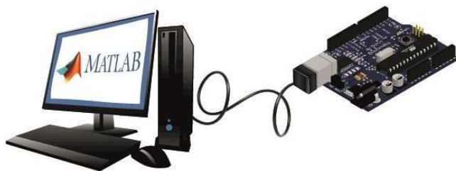
Figure 5. Representation of an Arduino card used to control the behavior of a system modelled in Matlab using a transfer function.
