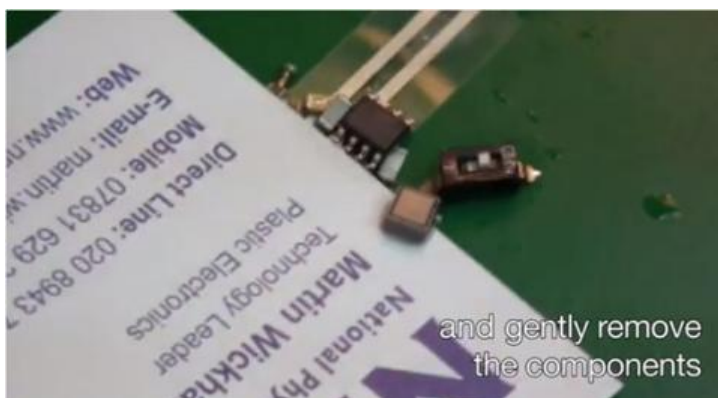
Figure 3. Removing components (Treacy, 2012)
