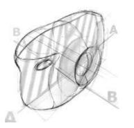
xii) Sketch over the construction geometry on an overlaid page connecting the sections and primitives.
