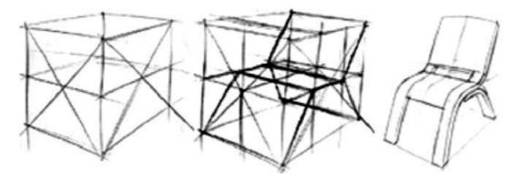
Figure 9. Stages in sketching a chair using crating.
