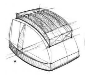
iii) The toast slot area is added by projecting upwards from the top surface of the quadrant sketch. A section is used to define the curve on the product sides at A.
