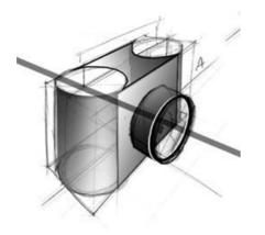
At this stage in the production of the sketch, crating and primitives have been employed to describe the geometry and proportions of the camera.
