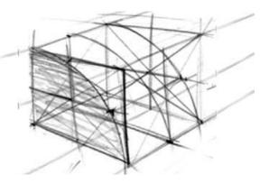
ii) The basic quadrant shape is roughed out within the crate.
