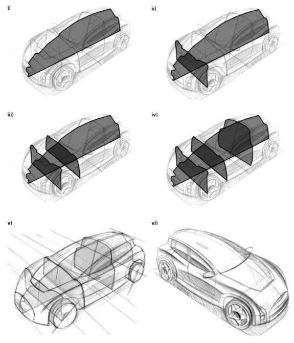
Figure 12. Using sections to sketch a car.
