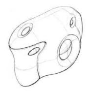
xiii) Tidy up line work and vary line thickness to describe form and component join lines etc.
